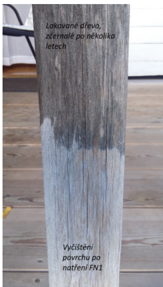
Temporary remediation restoration of damaged Wood: If you do not want to remove the harmed surface, both FN® NANO WOOD and low-cost FN®1 can be used to preserve and progressively improve (Fig. left).
