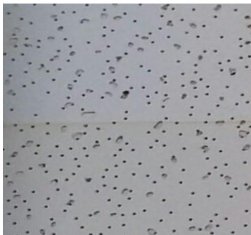
Fig.2 Ceiling plate painted in the upper half of the FN® paint. The experiment took place for 3 months in the smoking room and the surface was illuminated by UVA light.
