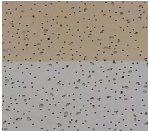
Fig.1 Ceiling plate painted in the upper half of the FN® paint. The experiment took place for 3 months in the smoking room and the surface has not been illuminated by UVA light.
